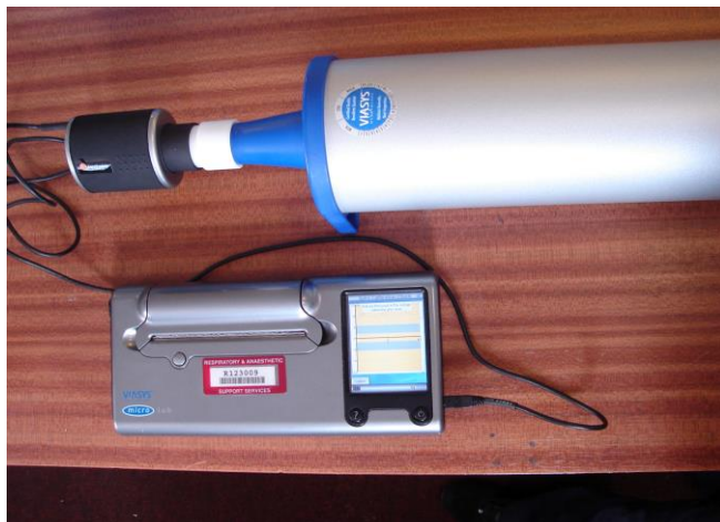
Figure 5: Calibration set up with 3L syringe
